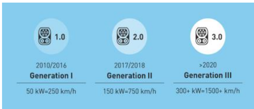
Figure 7: Increasing charging speed as announced by OEM's. The speed (km/h) indicates at what speed range can be added to the car when charging.
