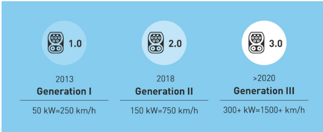
Figure 6: Increasing charging speed as announced by OEMs. The speed (km/h) indicates what range can be added to the car when charging.
